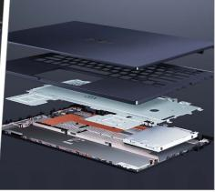
Rock Solid construction with alumnialloy lid, internal still bracing and proactive foam to protect HDD.
